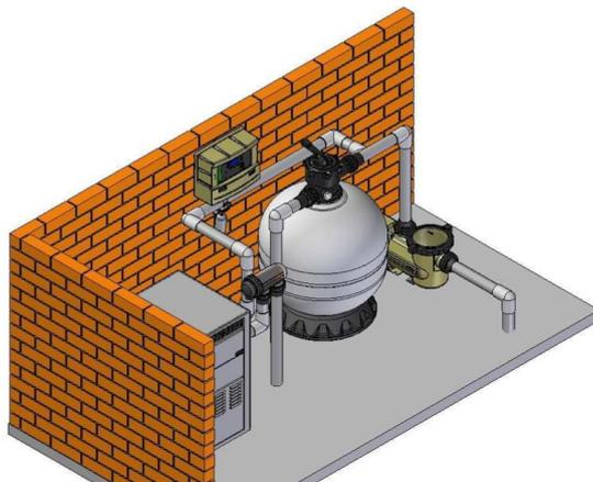
Once the Cell is located, connect the black multi-core cable to the cell. The green wire must be connected to the threaded terminal with the wing nut. The cable is designed to come from below the cell. Make sure wing nut are correctly tightened to ensure good contact.
